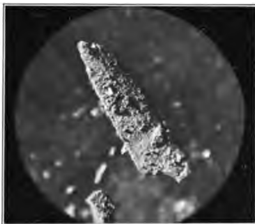
FIG. 41. — Photo-micrograph of a particle of crushed glass coated with nickel oxide (equivalent to 10 per cent of metallic nickel).
